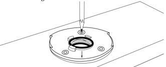
Figure 1-5. Marking Mounting Holes
