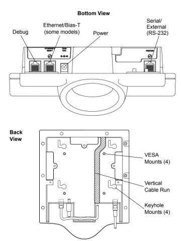
Note: Refer to the *MK 1100 Product Reference Guide* for installation and mounting procedures and Electrostatic Discharge (ESD) safe handling precautions.
